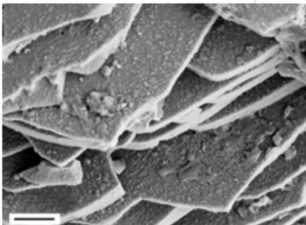
Scanning electron microscope view of the fractured surface of mother of pearl. The length of the bar corresponds to one micrometer.
