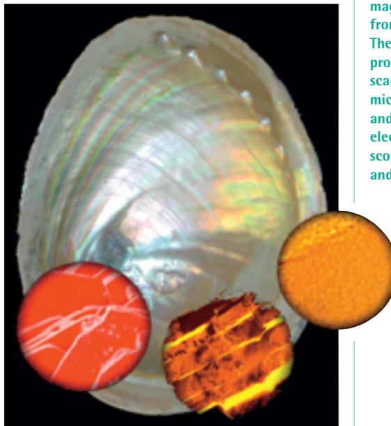
The shell of the abalone *Haliotis laevis*. The circles show detailed views of the structure of mother of pearl – with increasing magnification from left to right. The images were produced with a scanning electron microscope (red) and a transmission electron microscope (yellow and orange).
