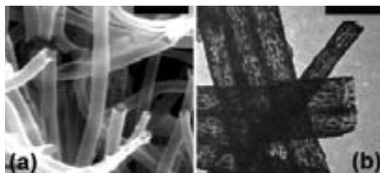
Fig. 1a: SEM image of the hollow titania fibers, b: TEM image of the tubes showing the mimicking nature of the sol-gel coating technique (scale bar is 5  $\mu\text{m}$ )
