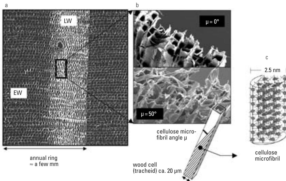
*Fig. 1: Hierarchical structure of wood. (a) Cross-section through the stem. Each annual ring is composed of earlywood (EW) and latewood (LW). (b) Fracture surfaces showing individual wood cells. The cell wall material is a composite of cellulose fibrils in a matrix of hemicelluloses and lignin.  $\mu$  is the spiral angle of the fibrils in the main cell wall layer. (c) Schematic representation of the crystalline structure of a typical cellulose fibril.*
