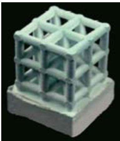
Fig. 2: Simple architecture made out of hydroxyapatite by rapid prototyping of the mould and subsequent gel casting (in collaboration with the Vienna University of Technology [13]). The strut thickness is close to the one of bone trabeculae (several hundred micrometers, see Fig. 3).
