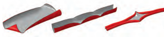
Fig. 4: Simulated rolling and folding of three actuating bilayers with different aspect ratios attached to a partially adherent substrate [9].
