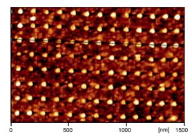
*Fig. 4: C60 aggregates on nano-patterned SiO<sub>2</sub>-substrate*
