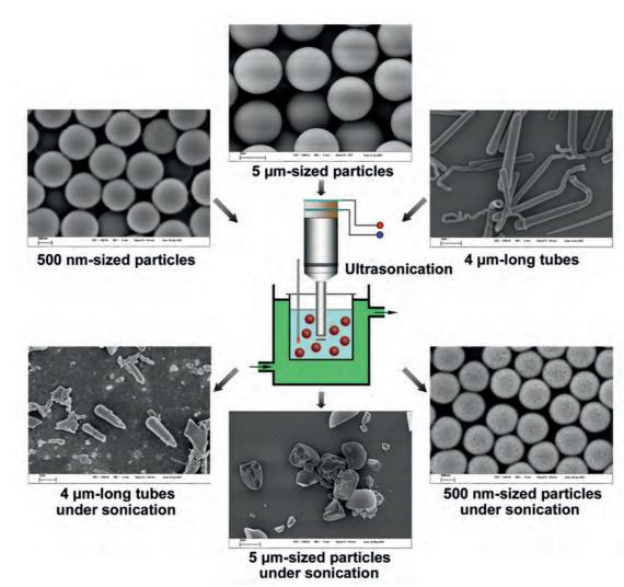
Figure 1: SEM Images of SiO<sub>2</sub> particles before and after ultrasonic treatment.
