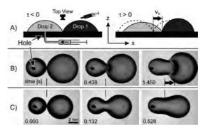
Fig. 4: A) Schematics of the experimental setup/procedure; B) non-coalescent twin drop movement (different, miscible liquids); C) instantaneous coalescence (identical liquids).
