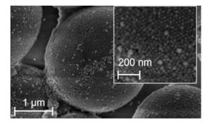
Fig. 1: SEM micrographs of silica-8-hydroxyquinoline composite containers based on Pickering emulsions [3].
