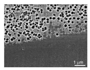
Fig. 2: SEM micrographs of the patterned AI sample after 10 min of sonication Upper part is the hydrophobized part [7].
