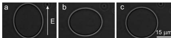
Fig. 1: A giant vesicle (phase contrast microscopy) subjected to an AC field of 10 V (2 kV/cm). The field direction is indicated with the arrow in (a). The external solution has a higher conductivity than the internal one ( \sigma_{in} > \sigma_{out} ). From (a) to (c) the field frequency increases causing shape transformations of the vesicle: (a) 5 kHz, prolate morphology; (b) 100 kHz, oblate shape; (c) 10 MHz, sphere.
