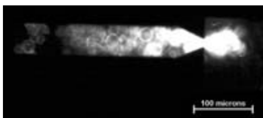
Fig. 2: Image demonstrating 20 \mu\text{m} capsules flowing through 10 \mu\text{m} constriction
