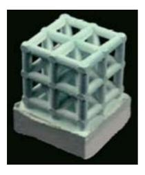
Fig. 2: Simple architecture made out of hydroxyapatite by rapid prototyping of the mould and subsequent gel casting (in collaboration with the Vienna University of Technology [13]). The strut thickness is close to the one of bone trabeculae (several hundred micrometers, see Fig. 3).
