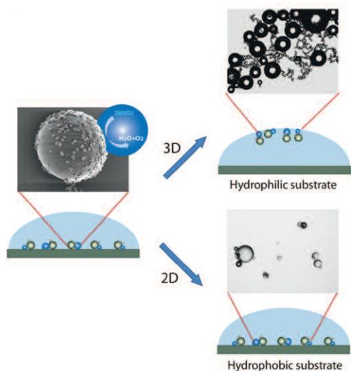
Fig. 8: Janus particles propelled by the formation of an oxygen bubble due to the splitting of  $H_2O_2$ . Increased hydrophobicity of the glass substrate changes the particle motion from three- to two-dimensional. [8]
