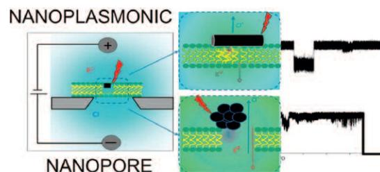
Fig. 2: Left: Schematics of a set-up to measure the conductance of a single channel in a membrane. Middle: Sketch of a nanorod or a nanoparticle aggregate with strong IR absorption to create local heating by light. Right: Single channel conductance/time traces. [3]
