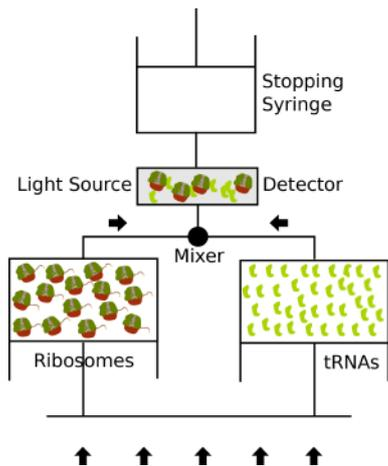
**Fig. 2:** Schematic drawing of a stopped-flow instrument to study translation by fluorescent probes. The syringe on the left is filled with a mixture of ribosomes and mRNAs, whereas the right syringe contains the tRNAs. Translation begins when both solutions are mixed. Progression of translation is monitored by a fluorescent signal emitted by fluorophores attached to the N-termini of the elongating peptides.
