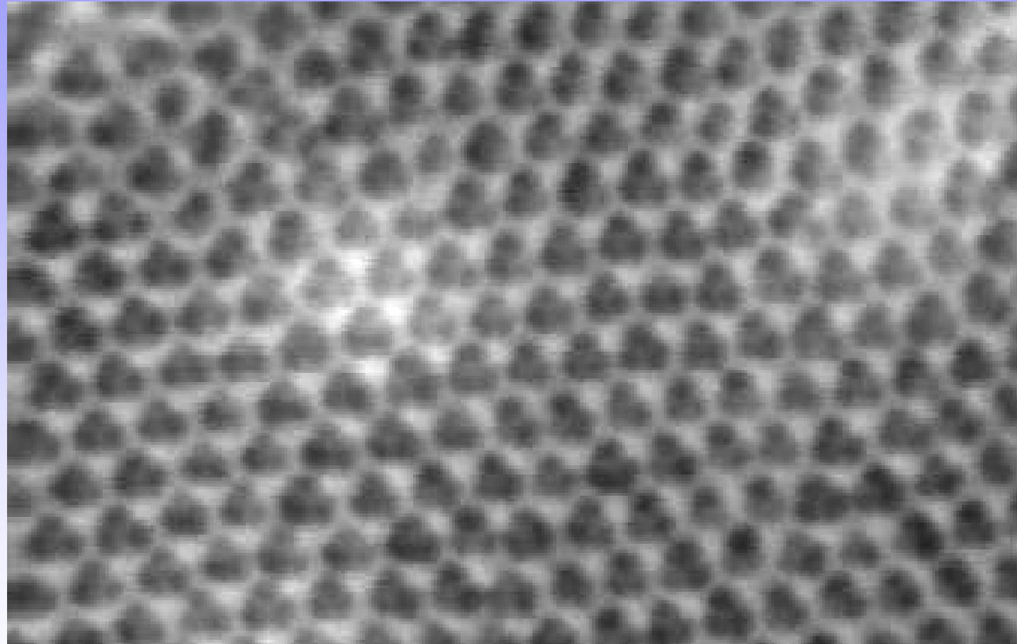
HR-SEM without contrasting: inverse opal structure with  $d \approx 15$  nm
