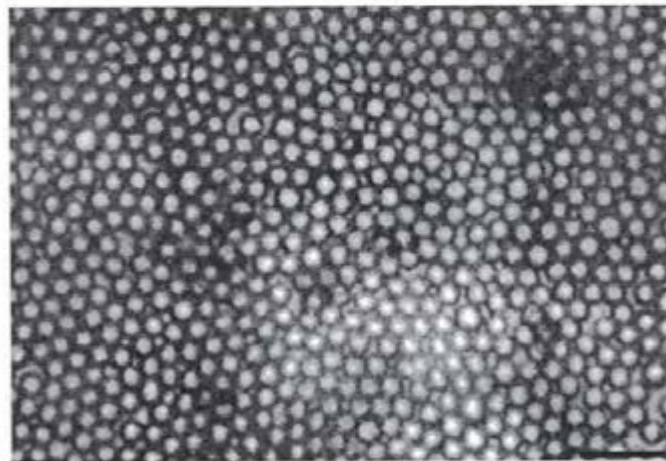
Figure 3. (upper) Optical microscope image of a single water-in-cyclohexane emulsion drop coated with 3.2 \mu\text{m} diameter hydrophilic latex particles ( \phi_w = 0.6 , 1 wt % in water). Scale bar = 50 \mu\text{m} . (lower) Enlarged portion of the water drop surface showing packing of individual latex particles. Scale bar = 15 \mu\text{m} .
