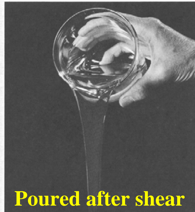
FIG. 10 Left thixotropic and right nonthixotropic solutions of CMC.
