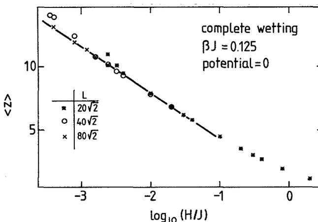
FIG. 3. Coverage  $\langle z \rangle$  for  $J/T \equiv \beta J = 0.125$  at the complete wetting transition ( $W_0 = 0$  and continuous  $z_i$ ) plotted vs  $\log_{10}(H/J)$ . The solid line is a fit to the asymptotic data. The deviations of the data from the fit curve at small  $H/J$  are due to finite-size effects (see Ref. 11).
