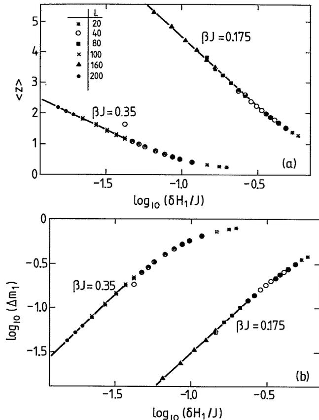
FIG. 1. (a) Coverage  $\langle z \rangle$  and (b) logarithm of excess surface order parameter  $\log_{10}(\Delta m_1)$  for model (1) at  $J/T = \beta J = 0.35$  and  $0.175$  (and  $H = 0$ ) plotted vs  $\log_{10}(\delta H_1/J)$ . The solid lines are fits to the asymptotic data described in the text.
