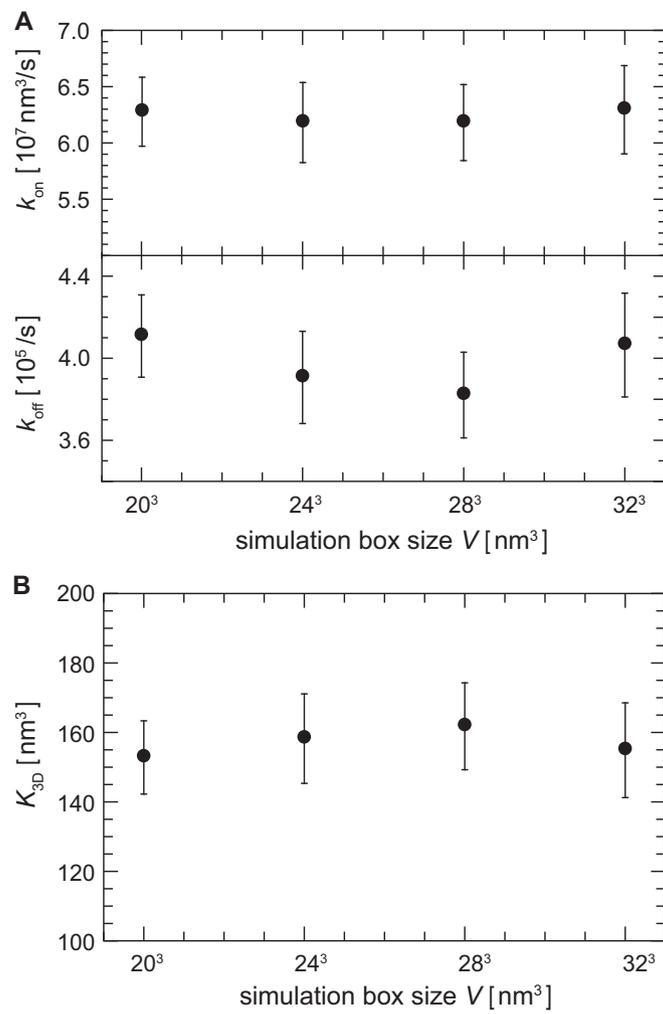
**Fig. S3.** (A) 3D on- and off-rate constants  $k_{\text{on}}$  and  $k_{\text{off}}$  and (B) binding equilibrium constant  $K_{3\text{D}} = k_{\text{on}}/k_{\text{off}}$  obtained from DPD simulations with a single soluble receptor and a single soluble ligand in cubic simulation boxes of different volume  $V$ .
