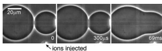
*Fig. 1: Snapshots from the fusion of two functionalized vesicles held by micropipettes (only the right pipette tip is visible on the snapshots). A third pipette (bottom right corner) is used to inject a small volume (few tens of nanoliters) of solution of  $\text{EuCl}_3$ , which triggers the fusion. The time after the beginning of the fusion process is indicated in the lower right corner.*
