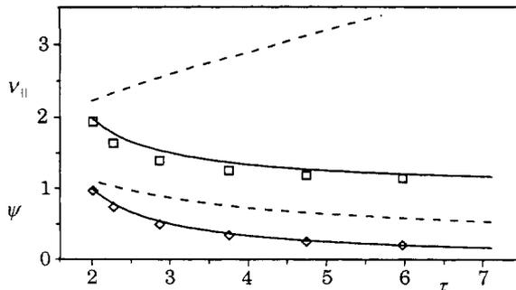
Fig. 4. – Critical wetting exponents for short-ranged potential. The numerical results ( $\square \nu_{\parallel}, \diamond \psi$ ) are compared with the predictions of the necklace model (NM) (—) and of the functional renormalization group treatment of an effective Gaussian model (FRG) (---).
