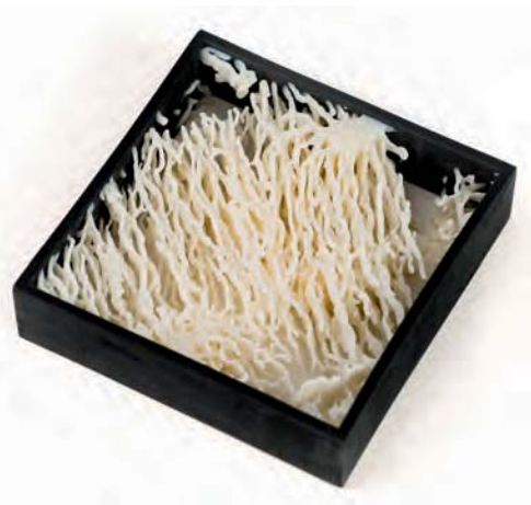
Model on request: Using rapid prototyping (right), a bone structure can be printed in 3-D. The scaffolds on which the researchers generate bone cells are formed using the same process (above).
