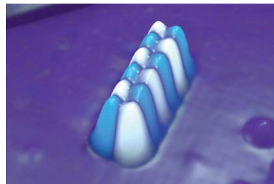
An atomic storage unit. Researchers from IBM and the Max Planck Society store one data bit in just 12 iron atoms on a copper nitride base. The alternating blue and white coloring illustrates the antiferromagnetic arrangement.
