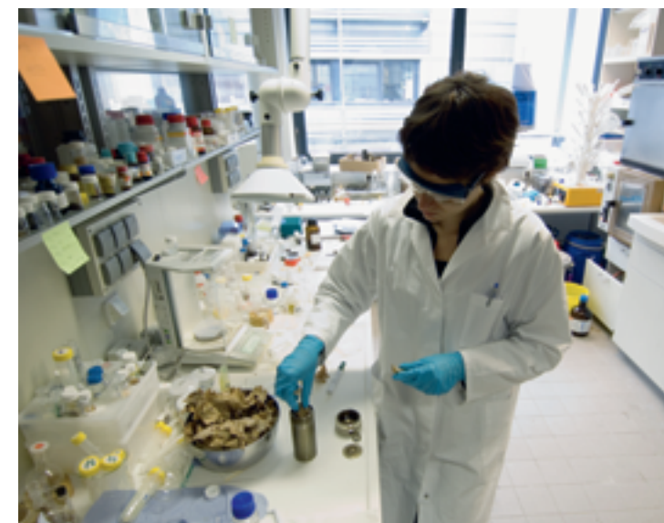
Put some biomass, such as greens, into a pressure container (left), add a couple of crumbs of a catalyst and heat it all up to 180 degrees Celsius in the absence of air: 12 hours later, out comes the black powder consisting of coal nanospheres (right).
