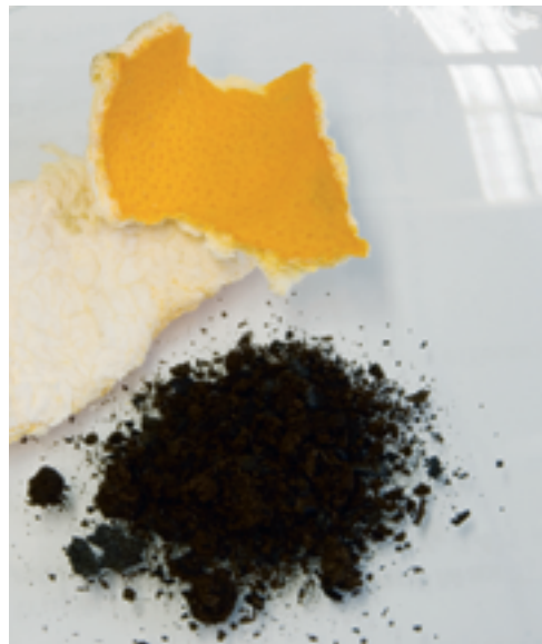
Hydrothermal carbonization in a pressure container turns biomass, such as orange peels, into extremely fine powdered coal (left). On the right is the inventor of the method, institute Director Markus Antonietti, with his colleague Anna Fischer.
