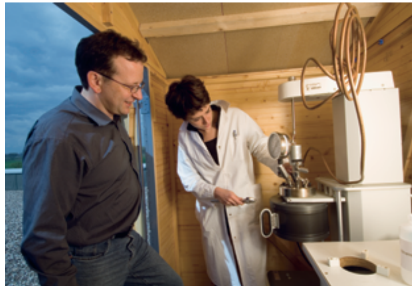
Hydrothermal carbonization in a pressure container turns biomass, such as orange peels, into extremely fine powdered coal (left). On the right is the inventor of the method, institute Director Markus Antonietti, with his colleague Anna Fischer.
