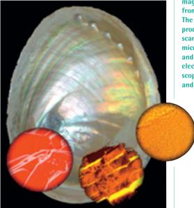
The shell of the abalone Haliotis laevigata. The circles show detailed views of the structure of mother of pearl with increasing magnification from left to right. The images were produced with a scanning electron microscope (red) and a transmission electron microscope (yellow and orange).
