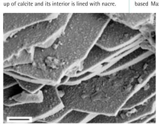
With the aid of high-resolution transmission electron microscopy and nuclear magnetic resonance spectroscopy, the materials researchers discovered that there is a very thin layer – just five nanometers (millionths of a millimeter) thick – of disordered calcium carbonate at the interface between the soft organic matrix and the aragonite
