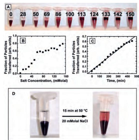
Fig.2: Poly (OEGMA-co-MEO<sub>2</sub>MA) capped gold NPs spontaneously transfer across the salty water-toluene interface.
