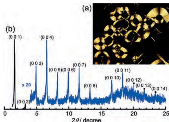
Fig. 5: Polarized optical micrographic texture (a) of mesophase of **2** at 190°C and the XRD patterns (b) indicating its long-range ordered lamellar organization.
