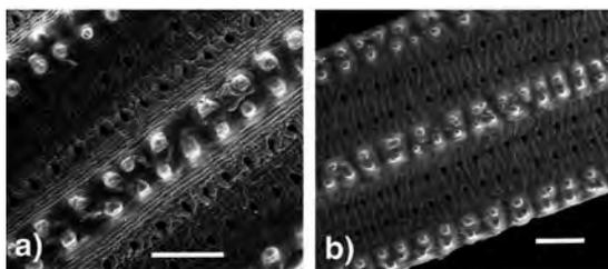
Fig. 3: Scanning electron micrographs of a native (a) and a long-term H<sub>2</sub>O<sub>2</sub> treated sample of *Equisetum hyemale* (b). The sample in (b) consists of pure silica (taken from [6]). The length of the bars is 300 μm.
