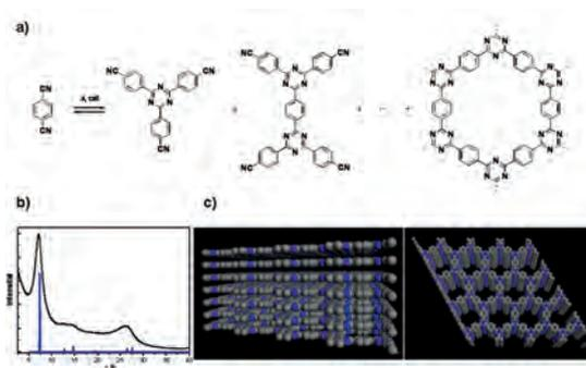
Fig. 4: a) Schematic presentation of the trimerization reaction of dicyanobenzene into a covalent triazine-based framework (CTF-1). b) Experimental (black) and calculated (blue) WAXS diffractogram of a triazine network made from 1,4-dicyanobenzene. c) Schematic representation of the structure of CTF-1.
