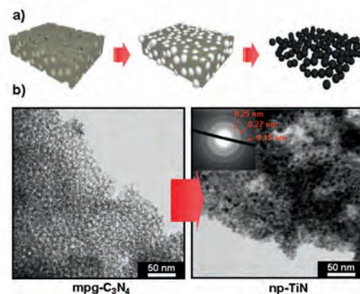
Fig. 2 a) Scheme of the "reactive templating" approach for the synthesis of metal nitride nanoparticles from mesoporous graphitic carbon nitrides b) TEM micrograph of  $mpg\text{-C}_3\text{N}_4$  and titanium nitride nanoparticles generated there from.
