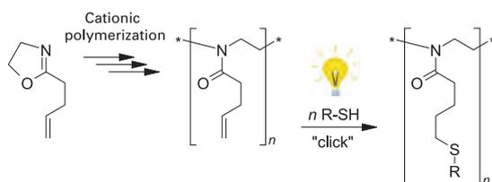
Fig. 1: Synthesis and click modification of poly[2-(3-butenyl)-2-oxazoline].
