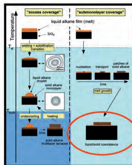
Fig. 1: Various alkane film topologies as a function of coverage and temperature. We find that this phase/topology diagram is generic and valid for many rod-like molecules. Currently our research activities focus on the equilibrium coexistence of monolayer domains and liquid film.
