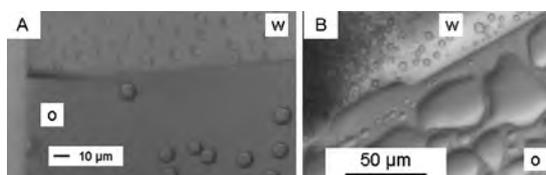
Fig. 1: Light microscopy images showing droplet formation on either side of the interface between A: chloroform – water and B: cyclohexane – water; o and w denotes the oil and water phase, respectively.
