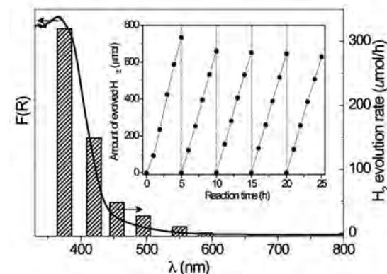
Fig. 3: Wavelength dependence of  $\text{H}_2$  evolution rate on Pt/ $\text{mpg-C}_3\text{N}_4$ . The inset is the stability test for Pt/ $\text{mpg-C}_3\text{N}_4$  under visible light irradiation (> 420 nm)
