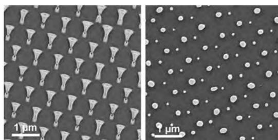
Fig. 5: Hexagonally arranged Au nanoshuttlecocks obtained by using bilayers of hexagonal close-packed PS spheres, etched by  $O_2$ -plasma for 25 min (left). Hexagonal binary arrays obtained by annealing the nanoshuttlecock arrays (right).
