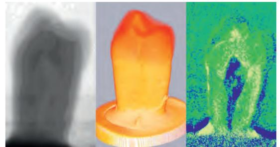
*Fig. 6: Neutron radiography (left) and reconstructed tomography (centre) may be used to directly visualize the changes in contrast due to exchange of D2O and MethD4. Differential image (right) produced by numerical subtraction, shows bright yellow areas where water attenuation values were higher in the 'wet' state as compared with dark green and blue areas where attenuation is higher in the dry state. Much of the asymmetric difference is seen in the root section of the tooth.*
