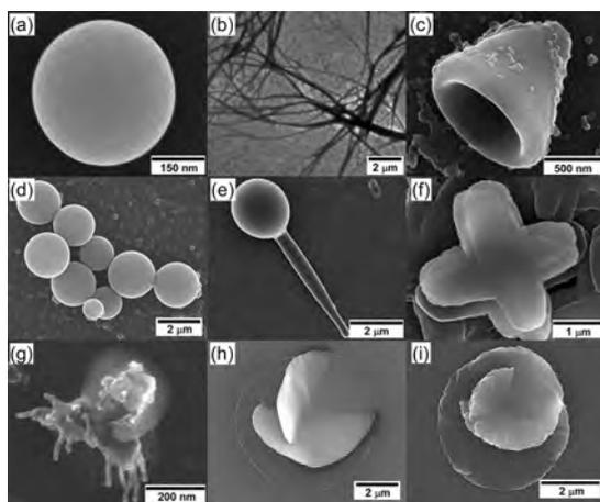
Fig. 1: SEM images of vesicles (a), fibrous (b), conical (c), micro-spherical (d), maracas-like (e), windmill-like sheets (f), jellyfish-like (g), left-handed (h) and right-handed (i) spiral objects of 1 obtained from various solvent conditions.
