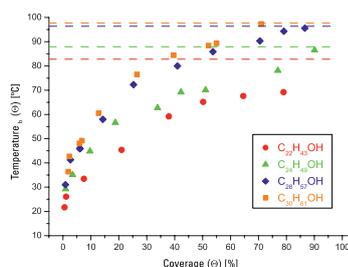
Fig. 3: Temperature of complete melting of long chain alcohol domains ( $T_b(\Theta)$ , see Fig. 2) as function of the coverage  $\Theta$  (in % of complete monolayers, dashed lines = melting temperature of a complete monolayer ( $T_b(\Theta=1)$ )).
