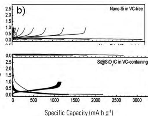
Fig.2: a) Silicon/carbon naocomposites showing core/shell morphology; b) Electrochemical performance of pure silicon nanoparticles (up image) in comparison with the carbon coated nanoparticles (down image) showing an improved cycling performance (60 cycles)
