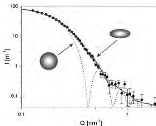
**Fig. 5:** Small-angle scattering profile (Intensity  $I$  vs. modulus of the scattering vector  $Q$ ) of the recombinant amelogenin rP172 at pH 8.1 and 4°C. The scattering is not consistent with monodisperse spheres (grey dotted line) but can be very well described by oblates (grey line).
