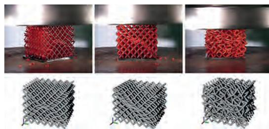
*Fig. 2: Strut architectures built by rapid prototyping (top) or in the computer (bottom). Mechanical compression leads to strain localisation that depends on the degree of disorder in the strut arrangement [6]*
