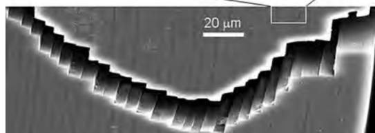
*Fig. 1: The driving force for a crack propagating in a multilayered material with periodically varying elastic modulus is vanishing close to the minimum of the modulus. The example above shows a layered bioglass spicule with a series thin protein interlayers (dark grey). The calculation is done for a modulus ratio of 6 between the stiff and the soft layers [4]. The arrow shows the propagation direction of the crack.*
