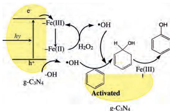
Scheme 1: The proposed coupling process of visible-light-induced redox catalysis with one-step phenol synthesis by  $\text{Fe-g-C}_3\text{N}_4$
