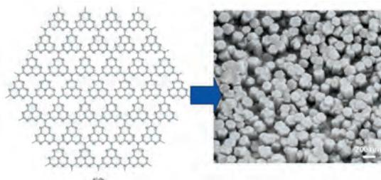
Fig. 1: The schematic internal structure of  $g\text{-C}_3\text{N}_4$  is reflected in the crystal morphology. SEM images of crystalline graphitic carbon nitride prepared in molten salt show hexagonal prisms.
