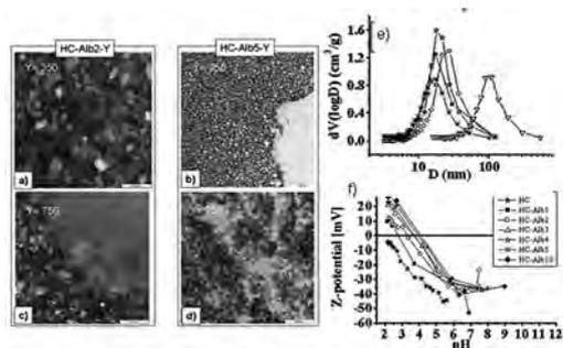
Fig.3: a) TEM micrograph of nitrogen doped carbon obtained from hydrothermal carbonization of glucose in the presence of a, b) 2% albumine; c, d) 5% albumine e) pore size distribution of the nitrogen doped materials showing their nanostructured character f) zeta potential measurements proving the positive charge of the materials at negatives pH due to nitrogen protonation
