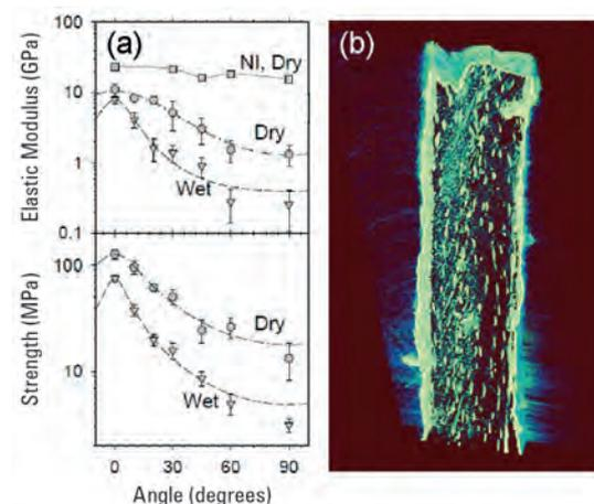
Fig. 2: High mechanical anisotropy of fibrolamellar bone packets as a function of angle to main fiber direction. A 3D X-ray microtomographic image of a bone packet is shown on the right.
