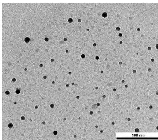
Fig. 4: TEM micrograph of boron carbonitride nanoparticles obtained after treatment for 6 h at  $1000^\circ\text{C}$  of a  $\text{C}_3\text{N}_4$  mesoporous matrix impregnated with  $\text{BH}_3$ -*tert*-butylamine.
