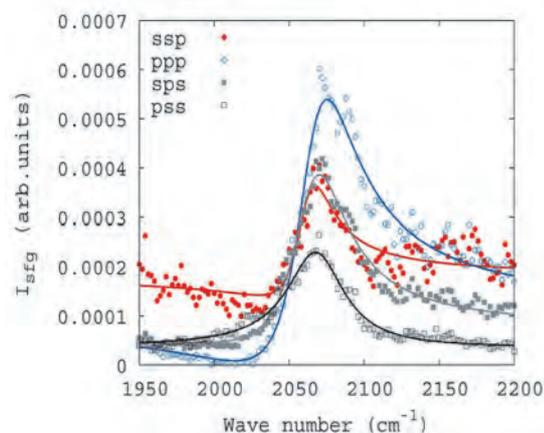
Fig. 2: Vibrational sum frequency spectra showing the CN stretch of the thiocyanate anion for 1 M potassium thiocyanate solution. The points and continuous lines represent the experimental data and fits respectively.
