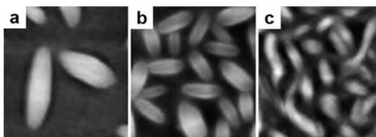
Fig. 5: SFM topography images ( $2.5 \times 2.5 \mu\text{m}^2$ ) of the ellipsoidal structures formed in solutions of polystyrene<sub>63</sub>-*block*-{poly( $\gamma$ -benzyl-L-glutamate)<sub>37</sub>}<sub>8</sub> in chloroform at different concentrations: a) 53%, b) 55%, c) 57%.
