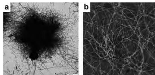
Fig. 2: (a) Transmission electron image of coagulate particles produced by poly(2-isopropyl-2-oxazoline) in pure water (scale bar = 2 μm). b) SFM topography image (10 × 10 μm<sup>2</sup>) of the coagulate formed under stirring in a mixture of water and tetrahydrofuran 98:2 (v/v) within 24 h at 65°C.
