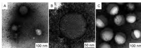
Fig. 2: TEM images illustrating the deposition of oligomeric particles onto styrene droplets during the early stage of unstirred emulsion polymerization; A:  $t_{\text{equ}} = 5 \text{ min}$  after 40 minutes polymerization time, B:  $t_{\text{equ}} = 120 \text{ min}$  after 30 minutes polymerization time, C:  $t_{\text{equ}} = 180 \text{ min}$  after 30 minutes polymerization time
