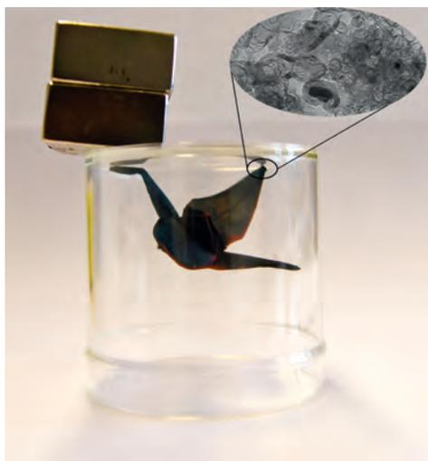
Fig.2: An origami (paper) crane previously soaked in a suitable iron salt solution then calcined, turns in a magnetic object (and thus attracted by a rectangular magnet, left) made of small  $\text{Fe}_3\text{C}$  nanoparticles embedded in a graphitic matrix (inset, right)
