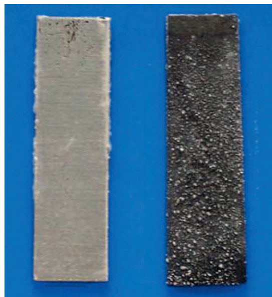
Fig. 1: Long term corrosion test: aluminium alloy covered by the polyelectrolyte/inhibitor coating (left) and unmodified aluminium plate (right).
