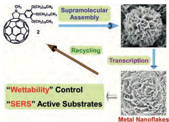
Fig. 4: Schematic illustration for the fabrication of metal nanoflake surfaces via supramolecular assemblies of a fullerene derivative ( 2 ) as template objects.
