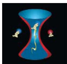
Fig. 1: FCS principle: Only molecules in the confocal volume are excited (left). The time correlation of the intensity spectrum (right) contains the information about the diffusion rates. The illustrations are reproduced from [1].
