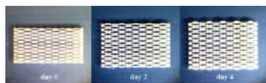
Fig 4. Swelling of a 3D printed honeycomb structure containing of transparent swellable and white non-swellable materials [9].
