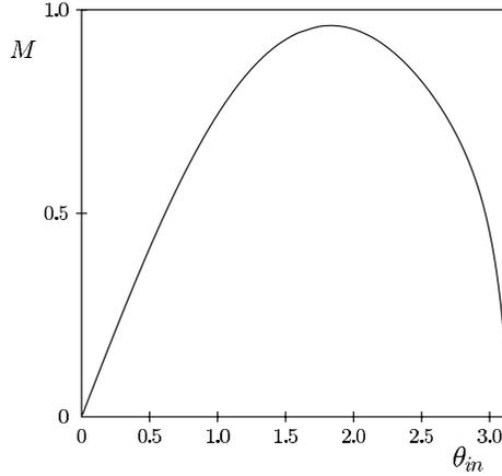
Fig. 3 – Mean curvature  $M$  of nodoid channel as a function of the interior contact angle  $\theta_{\text{in}}$  for ring-shaped surface domains with  $a_\gamma/a_\delta = 2$ .
