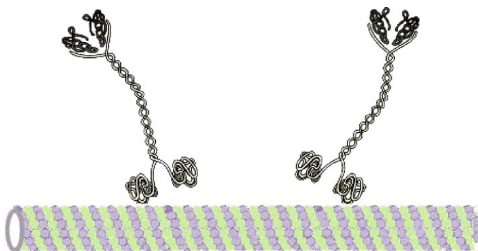
Fig. 1. Two kinesin motors (without cargo) bound to a microtubule segment. The microtubule is built up from tubulin dimers and has a diameter of 24 nm. Each motor molecule has two motor domains or heads which are connected by a neck region and a long stalk. The total length of the kinesin molecule is about 80 nm. Each motor head can bind to the microtubule and, in the bound state, adsorb and hydrolyze ATP.
