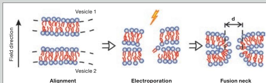
Fig. 1: Possible steps in electrofusion
