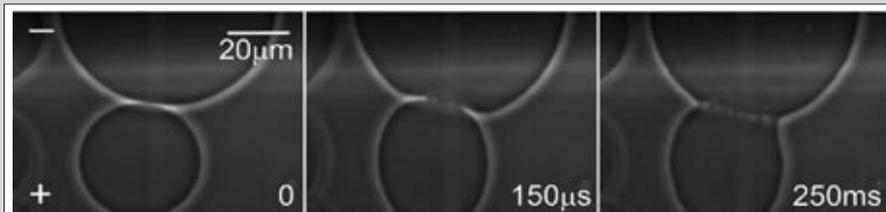
**Fig. 3:** Snapshot sequences of electrofusion of a vesicle couple. The time after the pulse start is indicated on each snapshot. First, the two vesicles were aligned via an applied A/C field (first snapshot). A D/C pulse (90 V, 150 µs) was then applied, which leads to fusion of the vesicles at several locations (second and third snapshots). The electrode's polarity is indicated with a plus (+) and a minus (-) sign.
